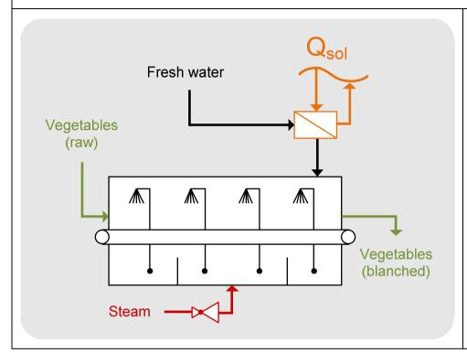
Example how to integrate solar heat for a blanching process in vegetable processing.
