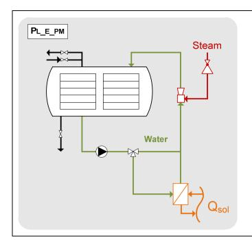
Example how to integrate solar heat for sterilization of canned food via autoclaves.
