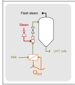
Example how to integrate solar heat for sterilization of milk (UHT Processing).
