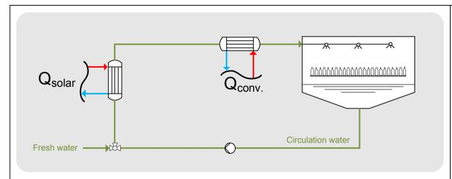
Example how to integrate solar heat for a tunnel pasteurizer.
