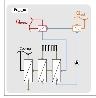
Example how to integrate solar heat for flash pasteurization.
